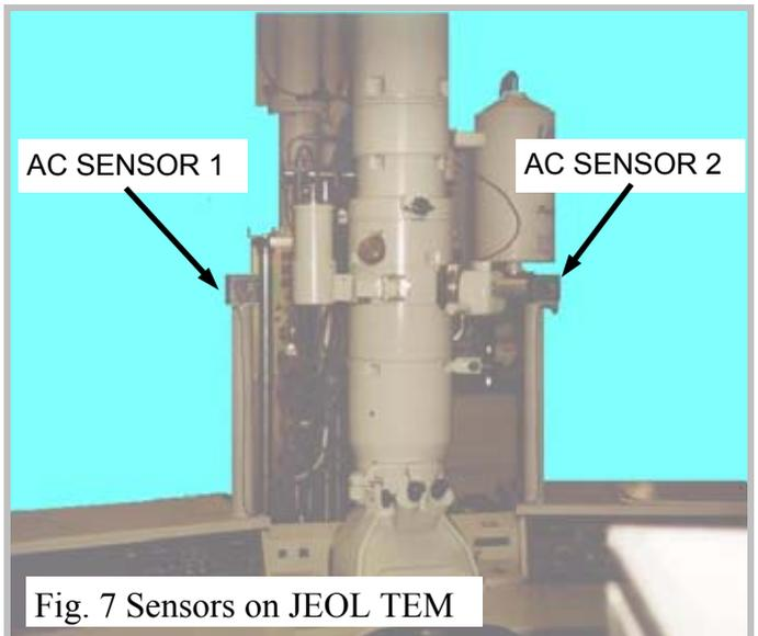
Fig. 7 Sensors on JEOL TEM
