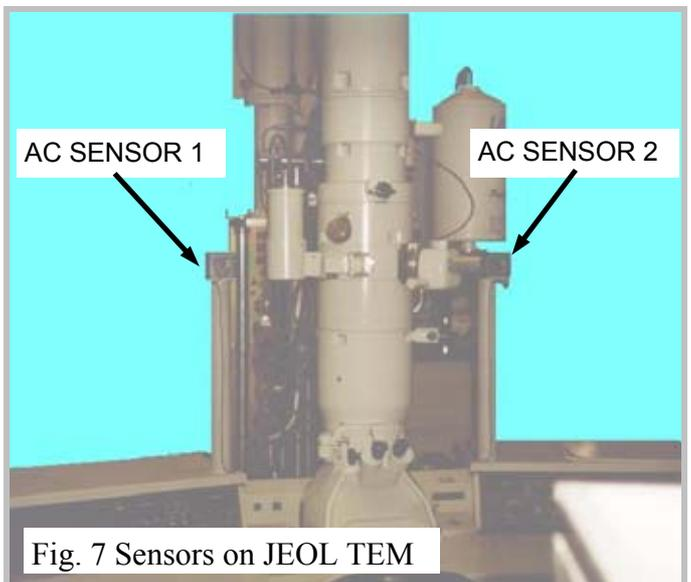
Fig. 7 Sensors on JEOL TEM
