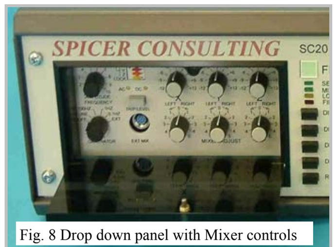
Fig. 8 Drop down panel with Mixer controls
