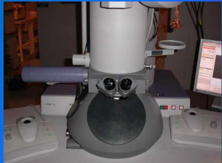
Every TEM (electron microscope) may produce ED patterns from individual single nanocrystals
